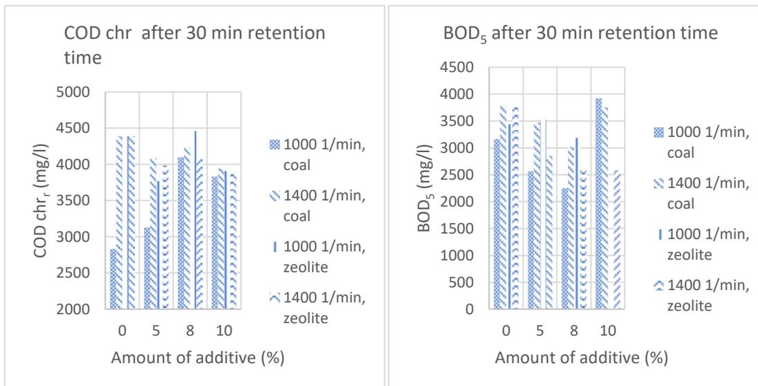
**Fig.6: Change in chemical oxygen demand (COD, left side diagram) and biological oxygen demand (BOD, right side diagram) ) due to the hydrodynamic treatment and using additives at various dosages, after 30 min retention time at different revolution numbers.**
