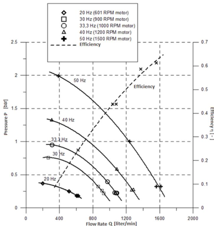
*Fig. 3: Pump characteristic curve [4].*
