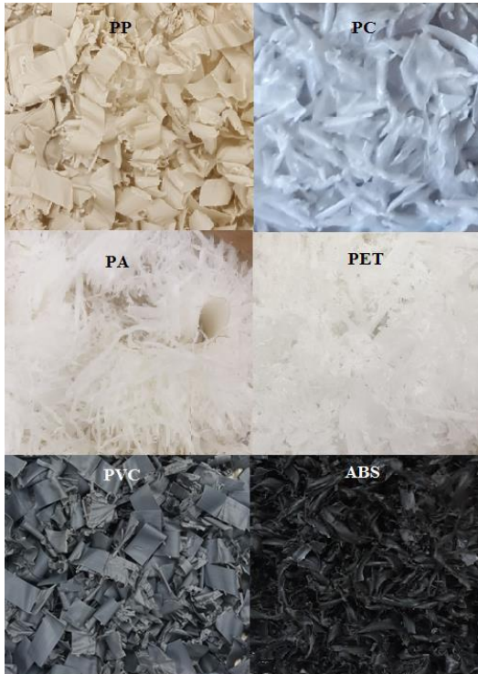
Figure 3. Samples after the turning machine process
