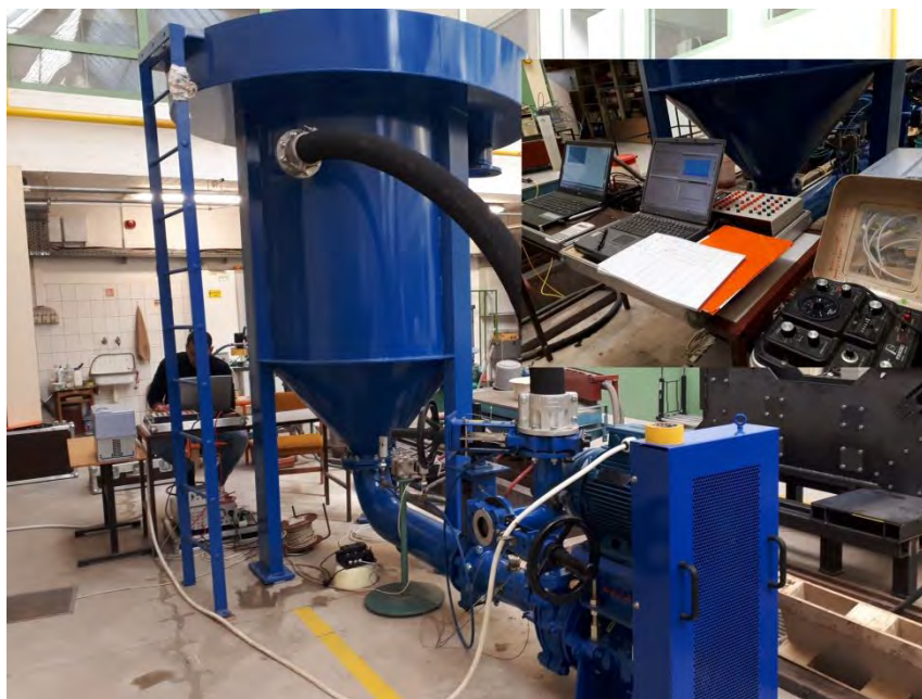
Fig. 2: Photo about the hydrodynamic experimental rig.
