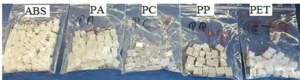
Figure 4. Samples which were used for the hammer mill experiment
