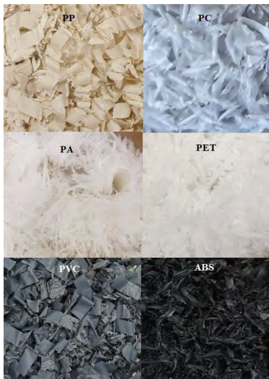
Figure 3. Samples after the turning machine process
